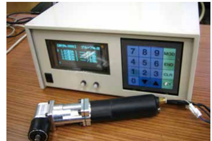
Double Guarantee Tightening (DGT) System Double guarantee of tightening torque by double torque sensors built in air tool
