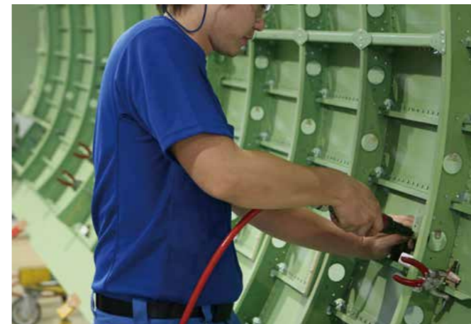
Air tool for assembling an aircraft which has realized very light weight and small size
