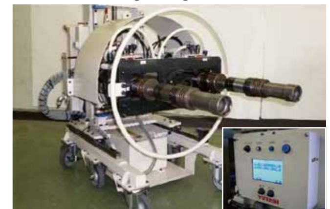
2-spindle nut tightening system for trucks and buses selected by "MONODZUKURI" New Selection in Kansai 2015
